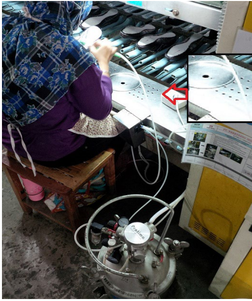
Figure 7 - Printing table with side exhaust
