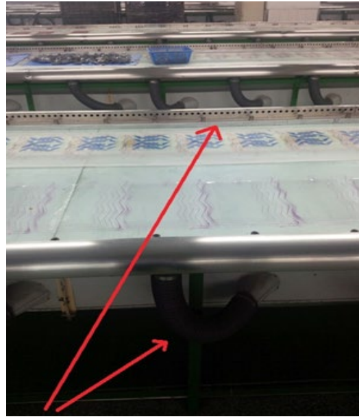
Figure 6 - Downdraft exhaust under adhesive applicator
