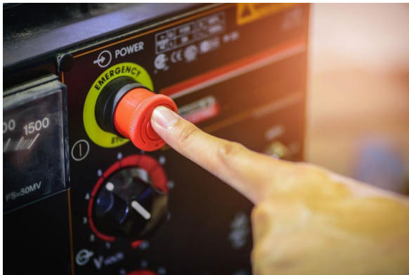
Figure 13 - Machine with Emergency Stop Switch.
