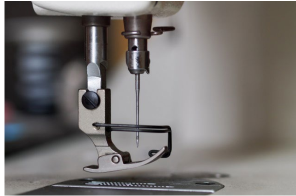
Figure 11 - Proper Needle Guarding on a Sewing Machine
