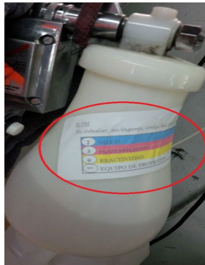
Figure 17 - Secondary Container Labeled with Hazards
